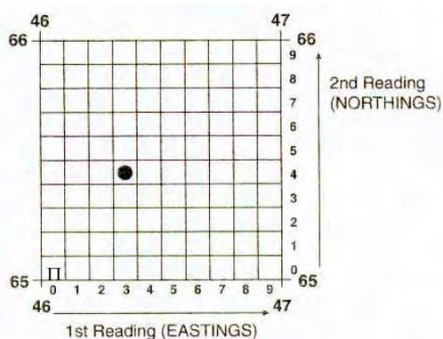
To give the six figure grid reference, first of all identify the grid square, in this case 4665. The third figure is obtained by dividing the space between grid lines 46 and 47 into ten equal parts. Similarly the sixth figure is obtained by a similar division of the gap between northings 65 and 66. This would result in a grid reference of 463654 for the dot and 460650 for the star. It should be noted that the first tenth is 0 and the last tenth is 9 in the divided grid square.
