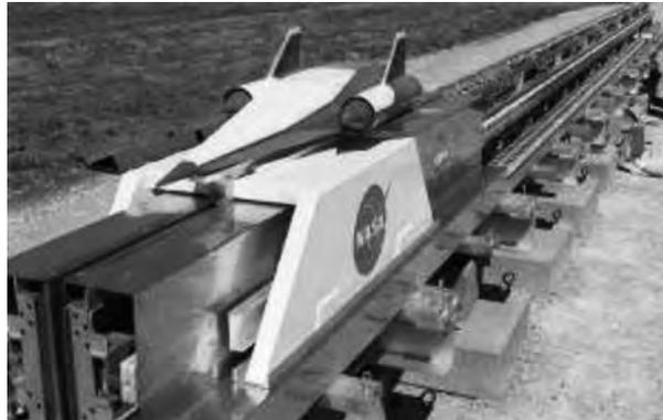
**Fig. E4.1** Photo: NASA tests a linear motor on a prototype Maglev railroad, 1999.
